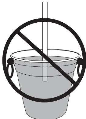
WRONG: Drain line is under water.
